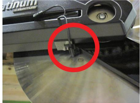
3. Place the sensor transmitter in a position where the pedals can not catch the wires. (we suggest to use the gap in the chain cover)
