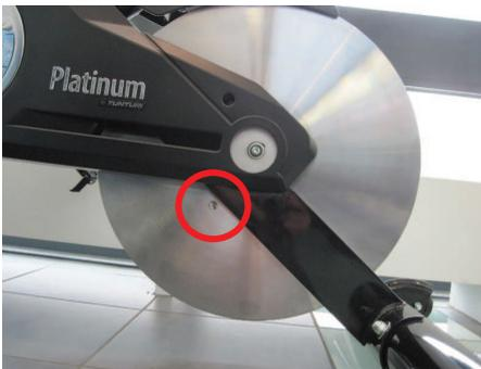
2. fit the sensor bracket to the chain cover in a position where the magnet passes for speed pickup. put the sensor in the holder.
